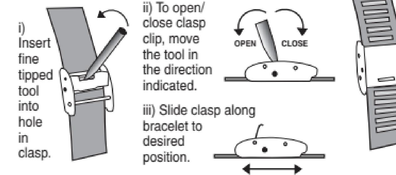
iv) When in selected position, locate tabs on back of clasp into slots on bracelet and snap down/close the clip [see procedure (ii)].
